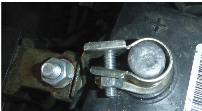
Cheap battery terminals are readily available and often installed poorly. Just because a cable end is new doesn't mean it was installed right or that the battery terminal under it was cleaned.
