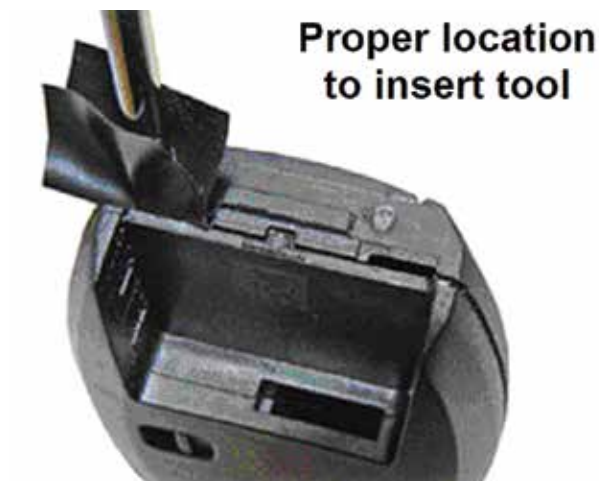
Remove the metal key insert, and use a plastic pry or electric tape-coated screw driver to separate the press-fit key halves.
