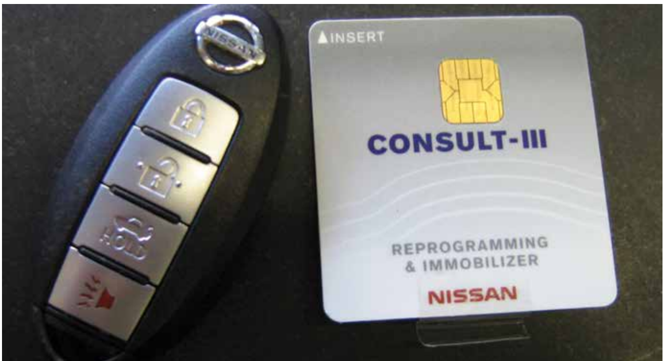
The CONSULT III plus will require an appropriate immobilizer unlock card to do work with Intelligent Keys.
