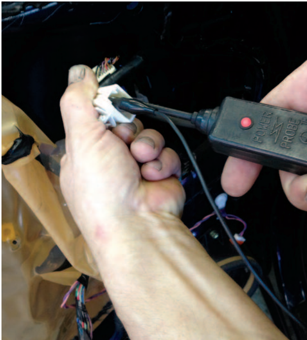
Jumpers and power probes are unnecessary and can cause damage.
