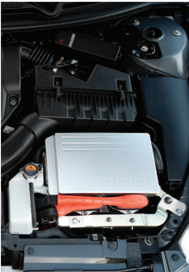
The 2007–2011 Altima Hybrid combines 244V technology and nickel metal hydride battery pack with a 2.5L Nissan internal combustion engine.
