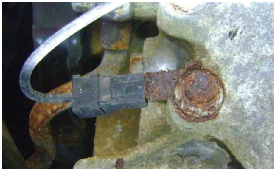
This Quest has been crippled by rust. After cleaning the mounting and replacing the terminal on the wire, it's time to check the rest of the grounds on the van for the same problem.
